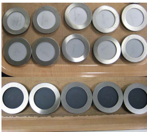
Figure 4. Electrolyte samples pressed into tablets for XRF analysis. First row- modified Rolseth device, second and third row- iron spatula.
